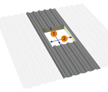
Saw a cut-out into the roof sheet:
