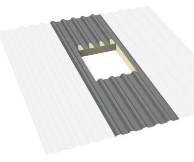
The ridges need an oblique sawing on top of the window hole (the right or left ridge stays, in case of a right or left laying panel).
